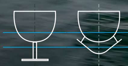
Typical cross section of hydrofoil-supported vessels: Fully submerged (left), Surface piercing (right)
