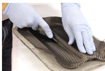
Figure: 4 consolidating into corners
