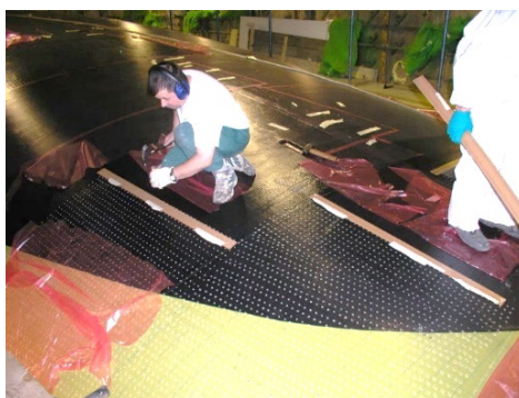
Figure: 6 Spiking Inner Skin to Vent Nomex.
